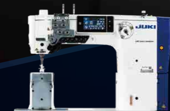
Semi-dry Direct-drive, Post-bed, Unison-feed, Lockstitch Sewing System with Vertical-axis Large Hook
